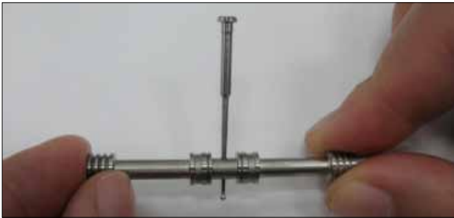
Figure 6: "Ball-in-Hole" Technology: Carbide ball extending through the hole in the spool
